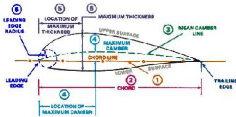
Figure 2. Standard Wing<sup>16</sup>
