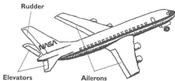
Figure 3. Control Surfaces<sup>17</sup>
