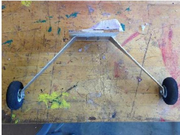
*Figure 13. Back Landing Gear*
