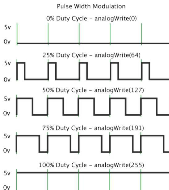
`analogWrite()`, allows a program to make use of the PWM function simply by plugging in a value ranging from 0 to 255, with the latter being the maximum possible
