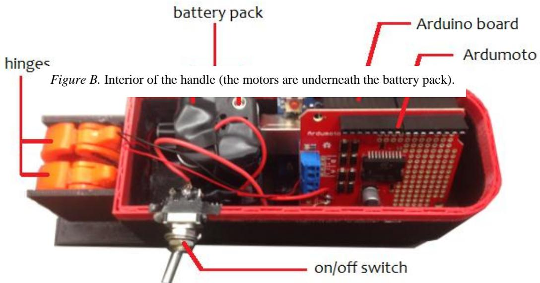
*Figure B.* Interior of the handle (the motors are underneath the battery pack).
