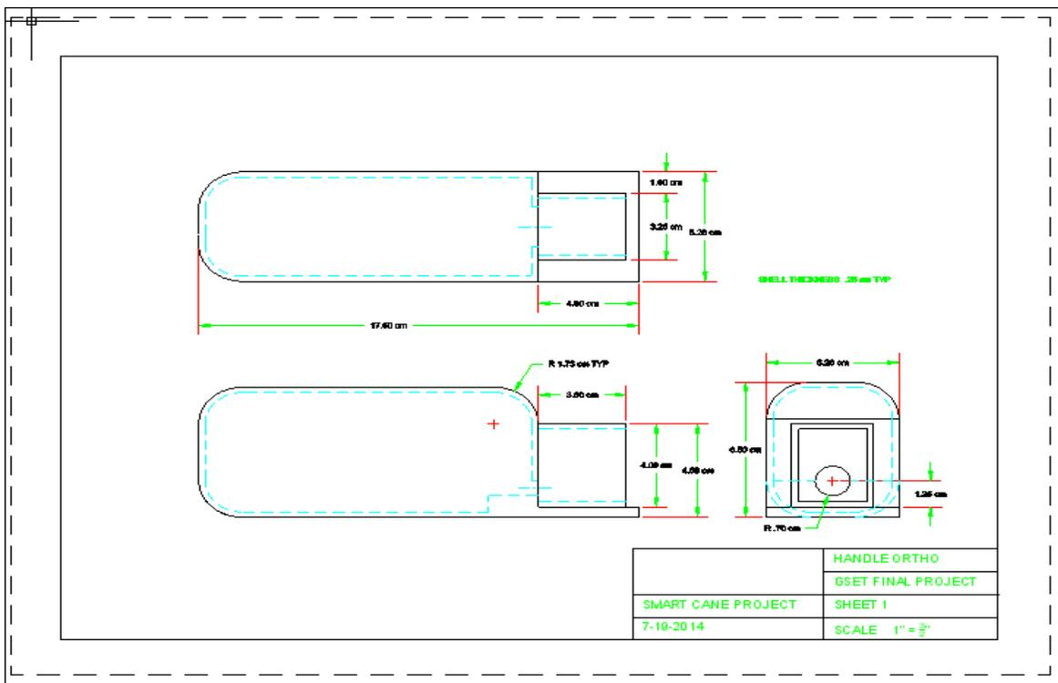
Figure D. Orthographic depiction of cane handle drawn using Autodesk AutoCAD
