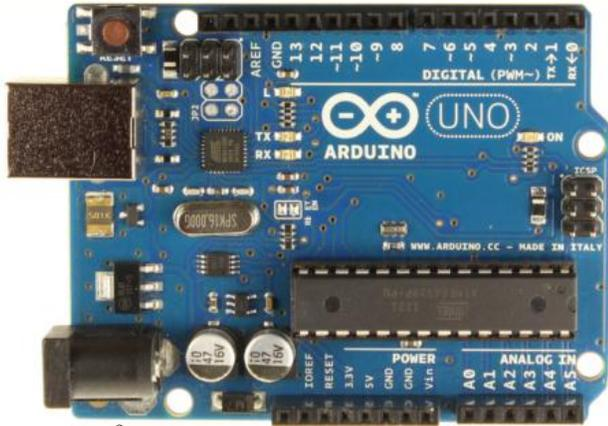
Figure 3.<sup>8</sup> *The Arduino Uno board. Digital pins, USB jack, (upper left), power jack (lower left).*
