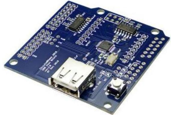
Figure 4. *The unassembled USB host shield.*<sup>11</sup>
