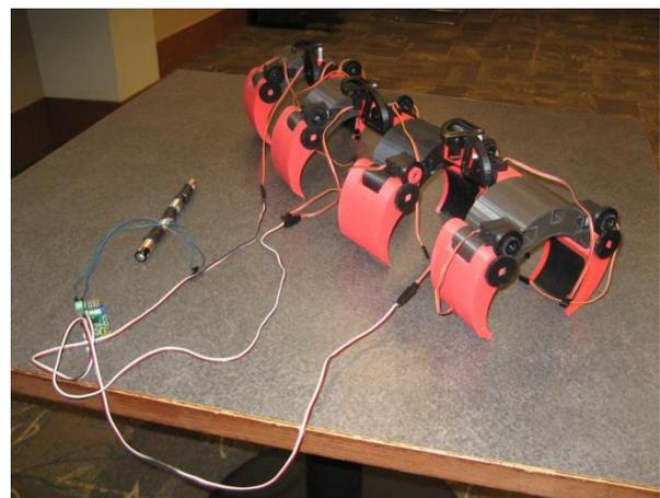
Figure 3: Mechanical Snake connected to the Pololu Mini Maestro 24 microcontroller
