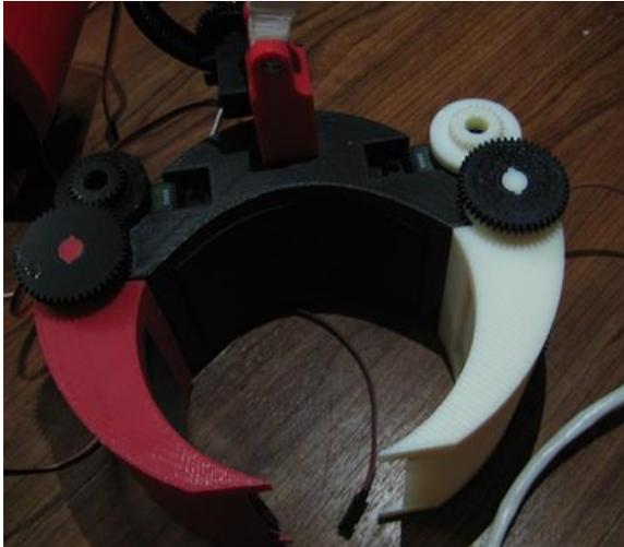
Figure 7: Repair; the white parts were reprinted and used to replace defective parts
