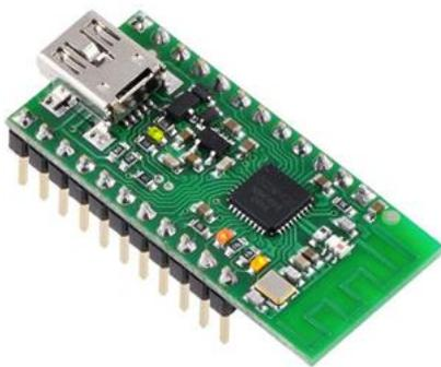
Figure 8: Pololu Wixel – wireless communication with the snake
