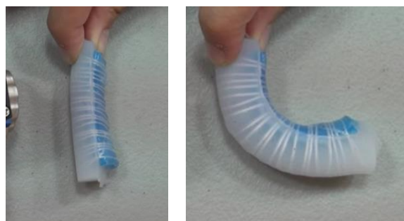
String-bound actuator. Left: just prior to actuation. Right: fully actuated.
