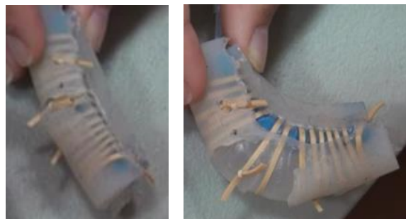
Rubber band-bound actuator. Left: just prior to actuation. Right: fully actuated.
