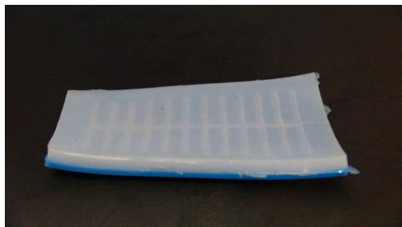
Original flat actuator. Air channels are oriented in a spine-like pattern throughout the actuator.
