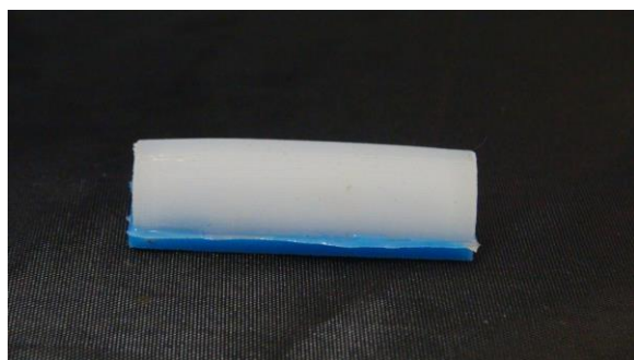
Straight actuator. A single air channel runs through the actuator in the longitudinal direction.
