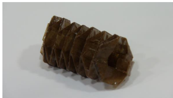
Octagonal prism-like origami actuator painted with Ecoflex. The balsa wood caps have not yet been attached.
