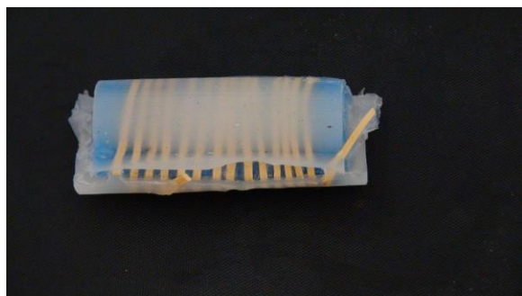
Rubber band-bound actuator. Improper curing caused the rubber bands to slide.
