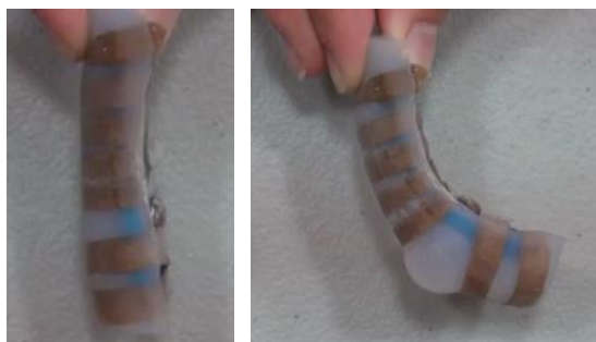
Paper-bound actuator. Left: just prior to actuation. Right: fully actuated.
