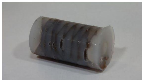
Octagonal prism-like origami actuator, submerged in Ecoflex. Air bubbles caused large holes that could severely weaken the actuator.
