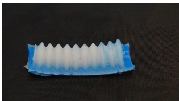
Sine actuator. Ridges along the top of the actuator allow the actuator to expand more easily in the longitudinal direction.
