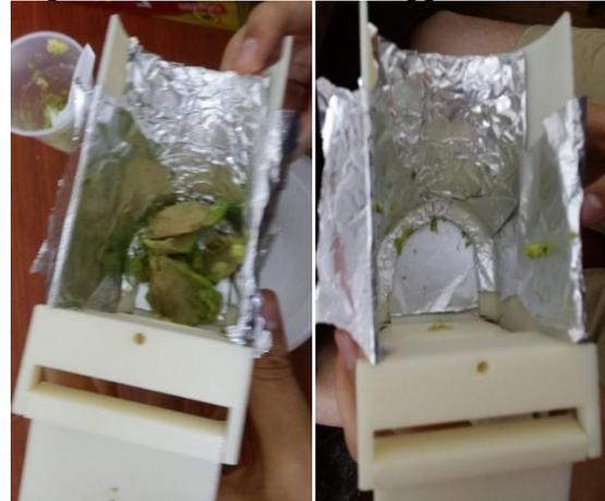
Figure 5. Right Angle prototype before and after the avocado test revealing a clean flush and latrine interior. The prototype was lined with tin foil prior to conducting the tests to keep the prototype clean, preventing avocado from staying behind in the ridges of the toilet's rough surface.
