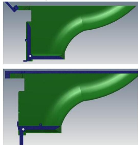
Figure 3. Right Angle design with open view, closed view
