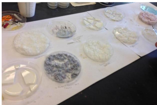
Figure 2: The ten Petri dishes after 50 hours of drying. From left to right: top row – (1) NaCl (low concentration), (2) CoCl<sub>2</sub> + NaCl + NH<sub>4</sub>OH, (3) HNO<sub>3</sub>, (4) NH<sub>4</sub>OH (low concentration), (5) CoCl<sub>2</sub> + NaCl + CaCl<sub>2</sub>; bottom row – (6) NH<sub>4</sub>OH (high concentration), (7) CoCl<sub>2</sub> + NaCl, (8) CaCl<sub>2</sub> (low concentration), (9) NaCl (high concentration), (10) CaCl<sub>2</sub> (high concentration)
