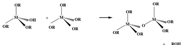
Figure 1: Hydrolysis and condensation diagrams<sup>5</sup>
