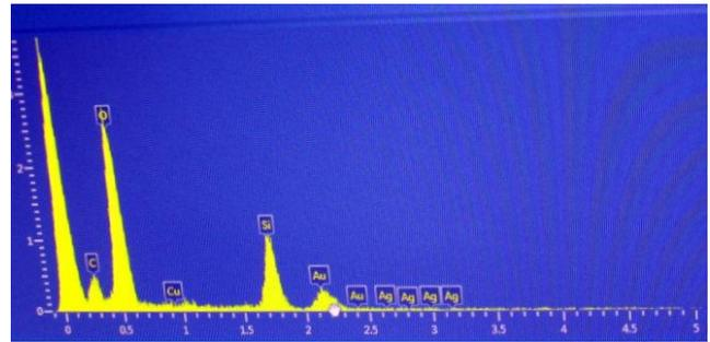
Figure 13: The composition of the acid-catalyzed gel
