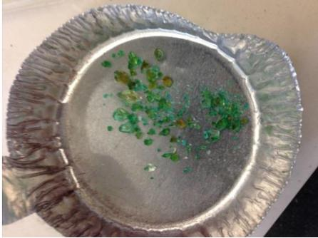
Figure 10: The dye-trapping abilities of the aged sol-gel
