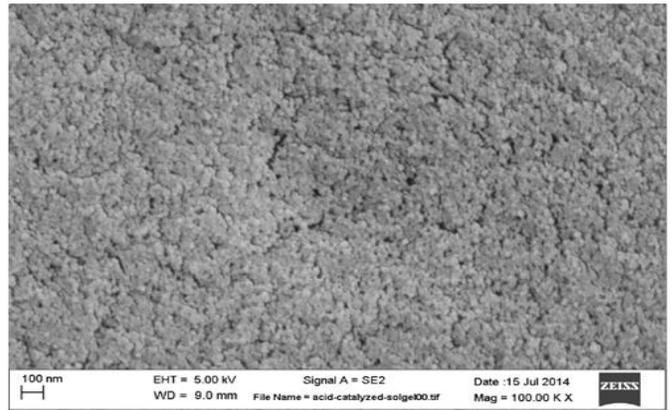
Figure 12: Scanning electron microscope image of an acid-catalyzed (HNO<sub>3</sub>) gel
