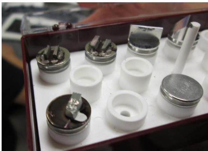
Figure 6: The samples of  $\text{NH}_4\text{OH}$  and  $\text{HNO}_3$  that were plated in gold
