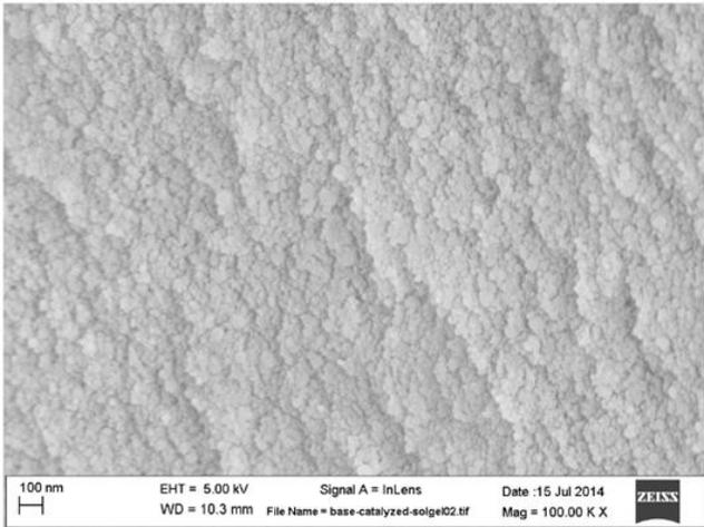
Figure 11: Scanning electron microscope image of a base-catalyzed (NH<sub>4</sub>OH) gel
