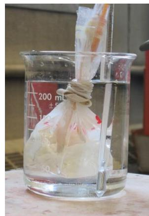
Figure 4: The set-up for taking the readings from the Heat Capacity Procedure
