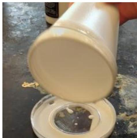
Figure 9: Using the small and large Petri dish combination to coat the rim of a Styrofoam cup
