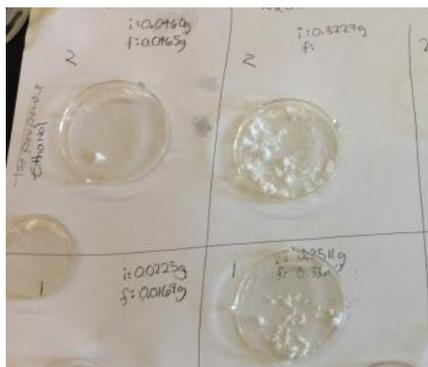
Figure 3: Samples of  $\text{NH}_4\text{OH}$ -catalyzed foam and  $\text{NaCl}$ -catalyzed foam in water and ethanol
