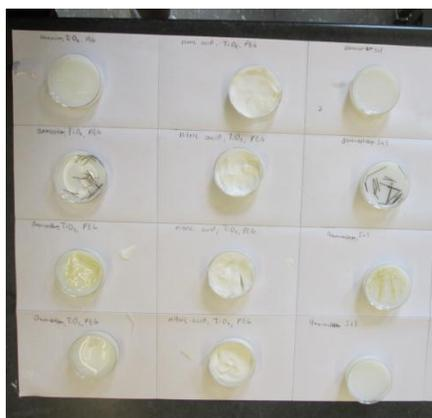
Figure 15: Dried samples from the third round of synthesizing gels by adding polymers
