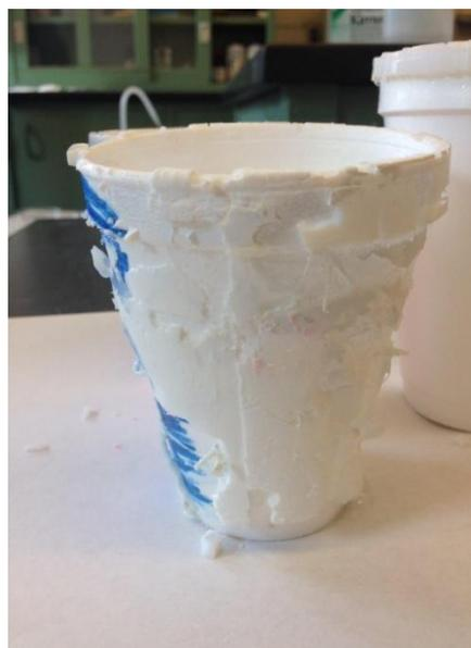
Figure 16: Styrofoam cup with absorbent rim and insulating coating
