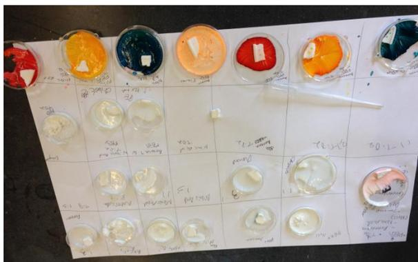
Figure 14: Dried samples from the second round of synthesizing gels by altering concentration and composition and adding dyes
