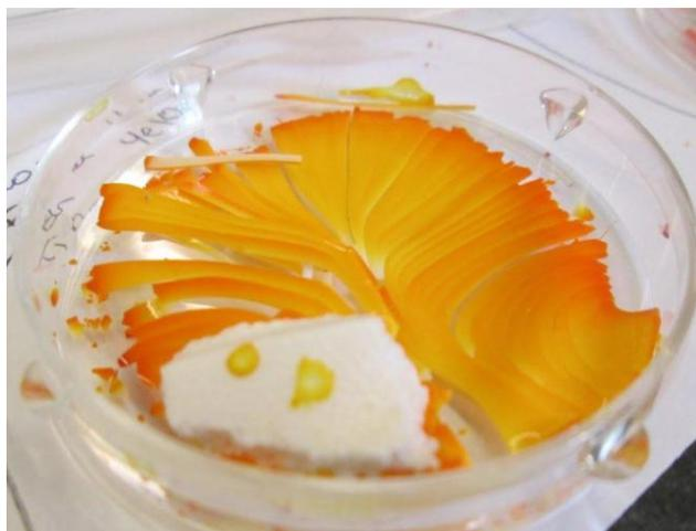
Figure 7: Sample from the second set of foam tests after 23 hours of drying.  $\text{NH}_4\text{OH}$ ;  $\text{TiO}_2$ , PEG, and Yellow Food Dye foam with a small piece of Styrofoam
